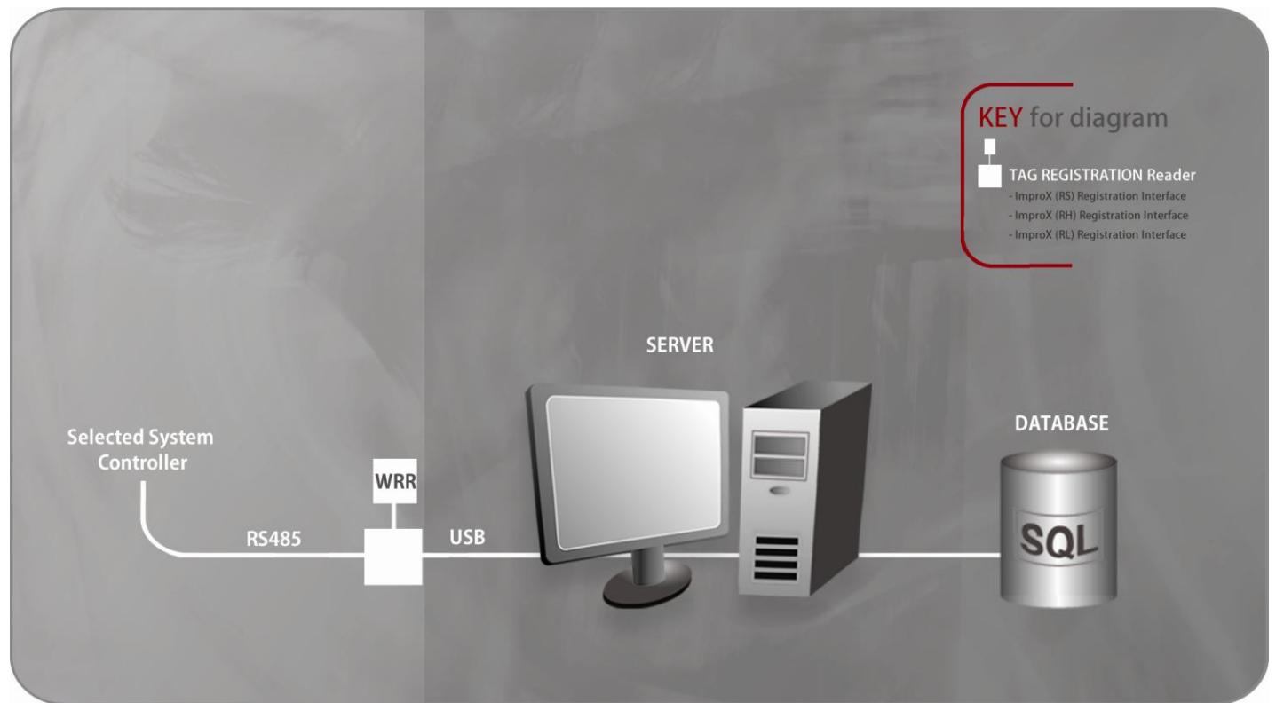
Figure 1: Wiegand Registration Reader Overview
